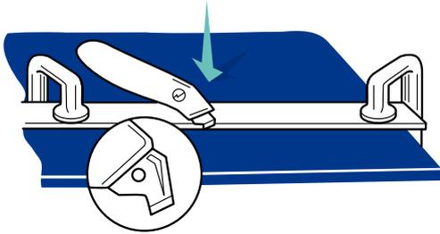
Figure 2 A Scribe-breaking Perspex® suitable for cutting Perspex®
