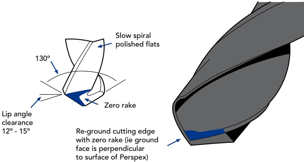
**Figure 3** A standard drill (130°) with cutting edges re-ground for use with Perspex<sup>®</sup>
